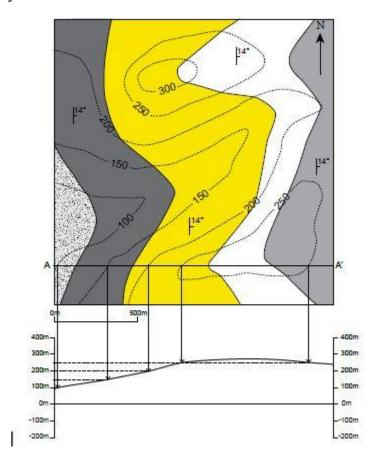
**Step 4:** Transfer the lithological boundaries, faults etc onto the cross section in the same way.
