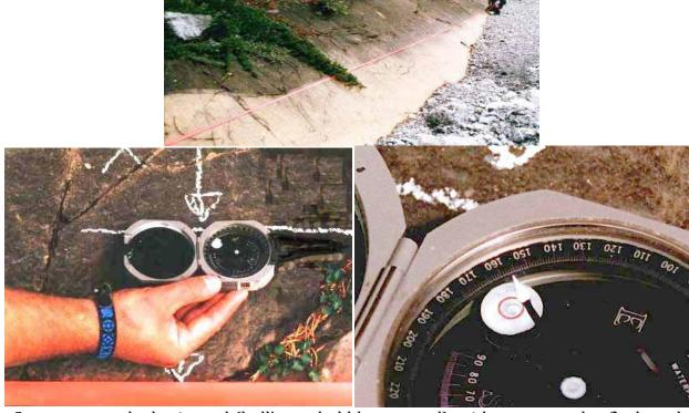
•Compass must be horizontal (bull's eye bubble centered), with compass edge flush to the tilted plane
